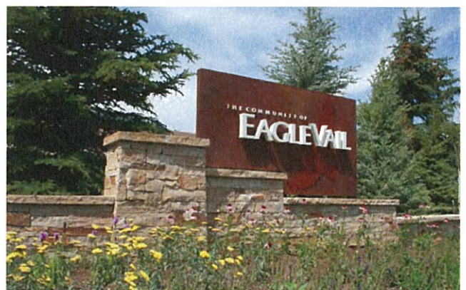
Image 34. Free standing signs shall be integrated with the ground plane through the use of plants and sign bases that anchor the sign to the site.
