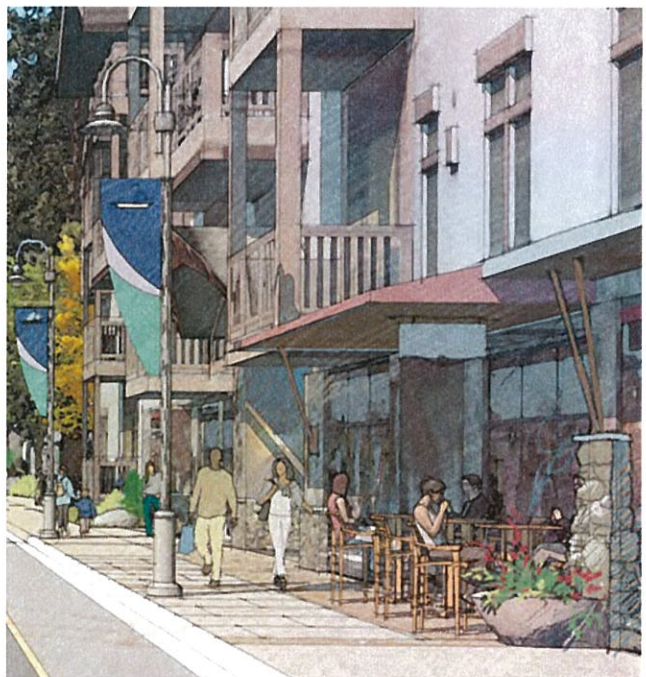
Image 15. Design elements such as increased setbacks and increased building articulation help create a comfortable zone for pedestrians.
